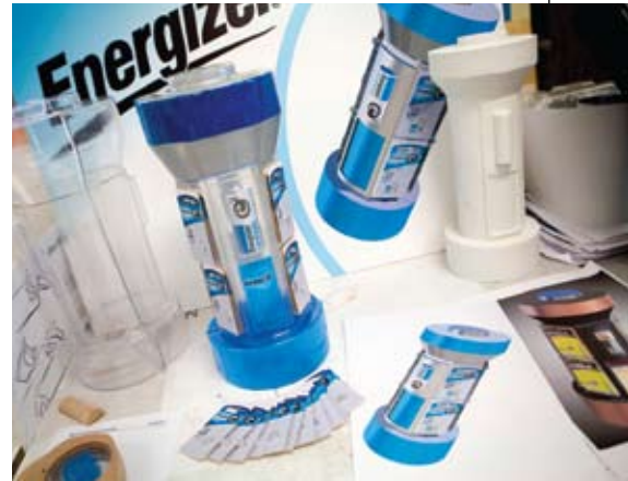
Eastman Chemical and Sheffield Plastics partnered with Auburn University to provide students with store fixture design training. The students worked with Vivak sheet to thermoform and bend the material into P-O-P designs.
